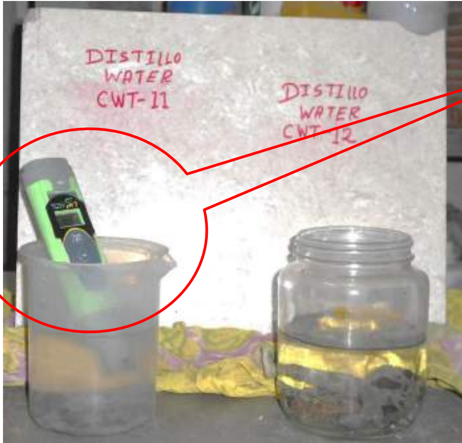
Concrete pH Test
