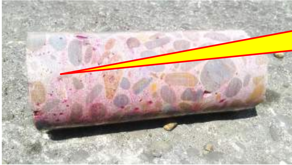
Carbonation Test with 0.2 % Phenolphthalein Solution
