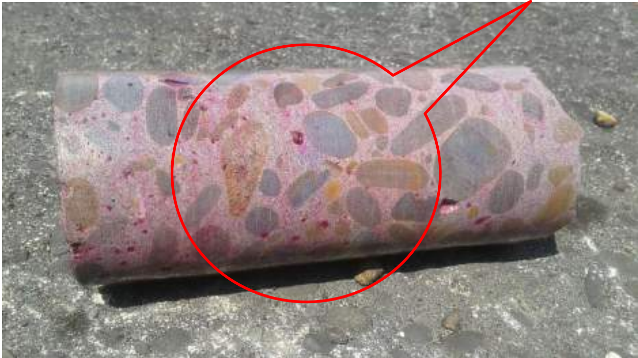
Concrete Carbonation Test with 0.2 % phenolphthalein solution
