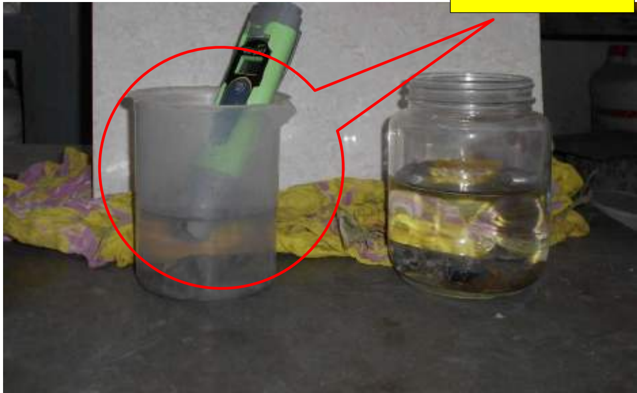
pH Testing of Concrete
